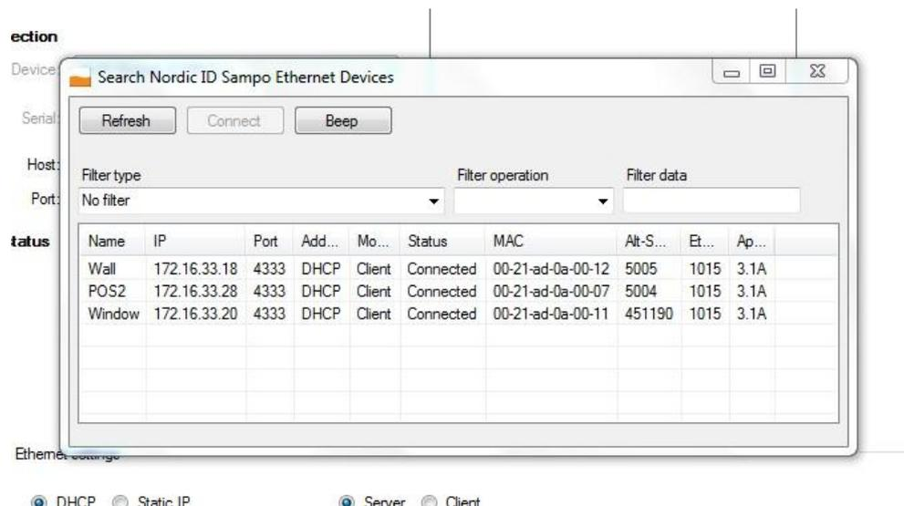
Select the RFID Reader from the list you want to connect and press the 'Connect' – button.
