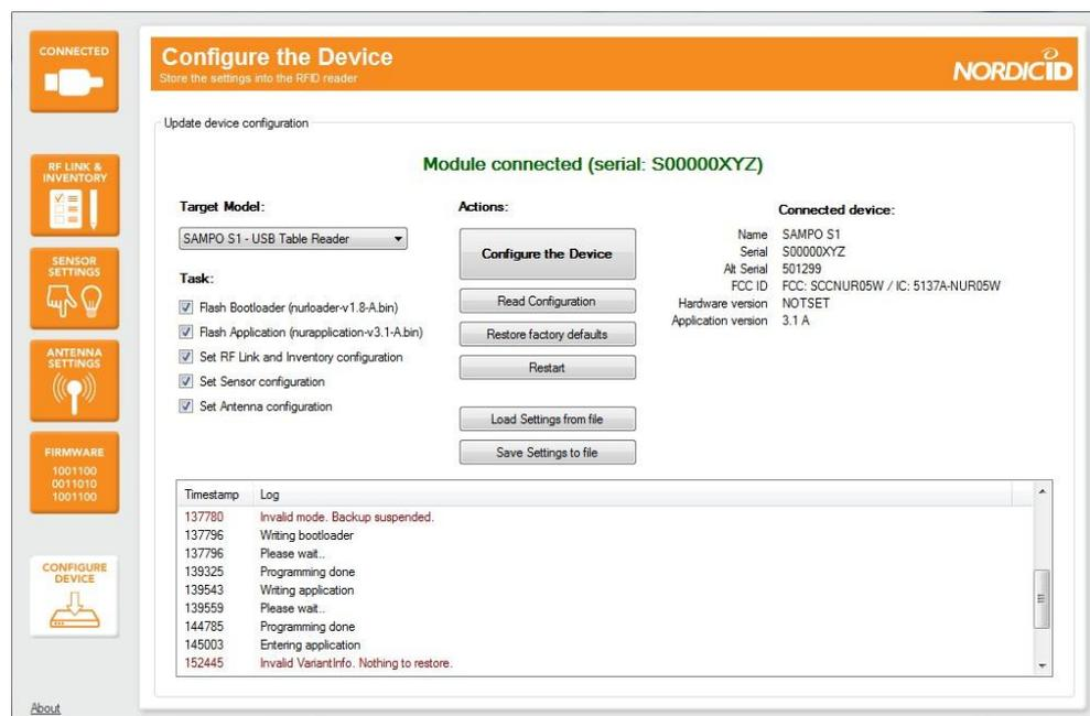
**Target Model:** This shows the model of the RFID reader which is connected to the configuration software.
